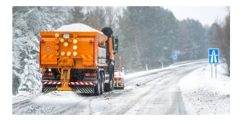
In freezing temperatures, specially designed trucks spread salt mixtures on roads and sidewalks to prevent accidents. The salt melts any snow or ice that is already on these surfaces, and also prevents water from turning into ice. This is because added salt lowers the freezing point of water.
