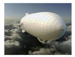
Unlike a balloon, a blimp has a shape and structure that enable it to fly and maneuver. The main part of a blimp is called the envelope. The envelope is the large bag that holds the gas, in this case, helium. The envelope is generally cigar-shaped, for aerodynamic purposes, and made of a durable airtight, lightweight fabric that is much like the fabric of a space suit. Since blimps are comparably light, they are much more fuel efficient that jets and other aircraft.
